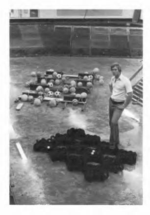
Plate 3. One-quarter scale model of TF-Breakwater in drained wave tank at Canada Centre for Inland Waters (model of Goodyear Breakwater in foreground). waves, but machine-generated and wind-generated wave spectra were also investigated. In the case of irregular waves, the transmission coefficient  $C_t\approx H_t/H$  and wave steepness H/L were evaluated using the peak-energy wave length and the average wave height as obtained from time-series analysis of the water surface elevation.
