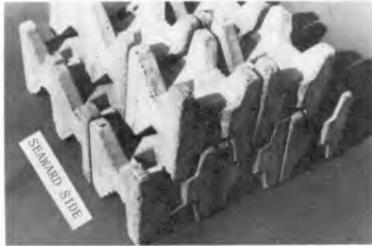
Fig. 5.- N-Shaped Blocks in Two Layers
