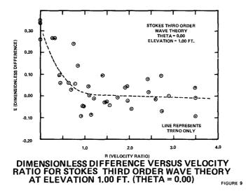
only the drag force is present. The coefficients of drag were determined by three methods. The first method used simultaneous measurements of the horizontal fluid force and velocity.
