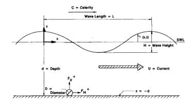
DEFINITION SKETCH OF THE PIPELINE PROBLEM FIGURE 1 configuration may represent a pipeline resting on the ocean bottom. The cylinder has both horizontal and vertical forces acting on it due to the passing wave and current. Only the horizontal drag force is investigated in this research.
