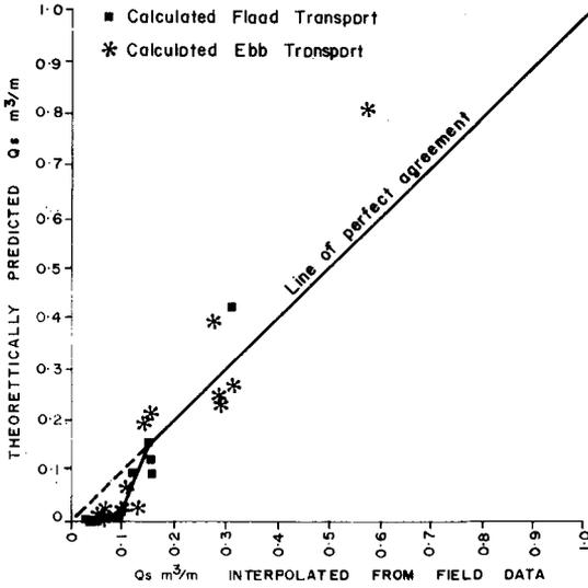
Figure 12 Comparison of Calculated and Measured Transport
