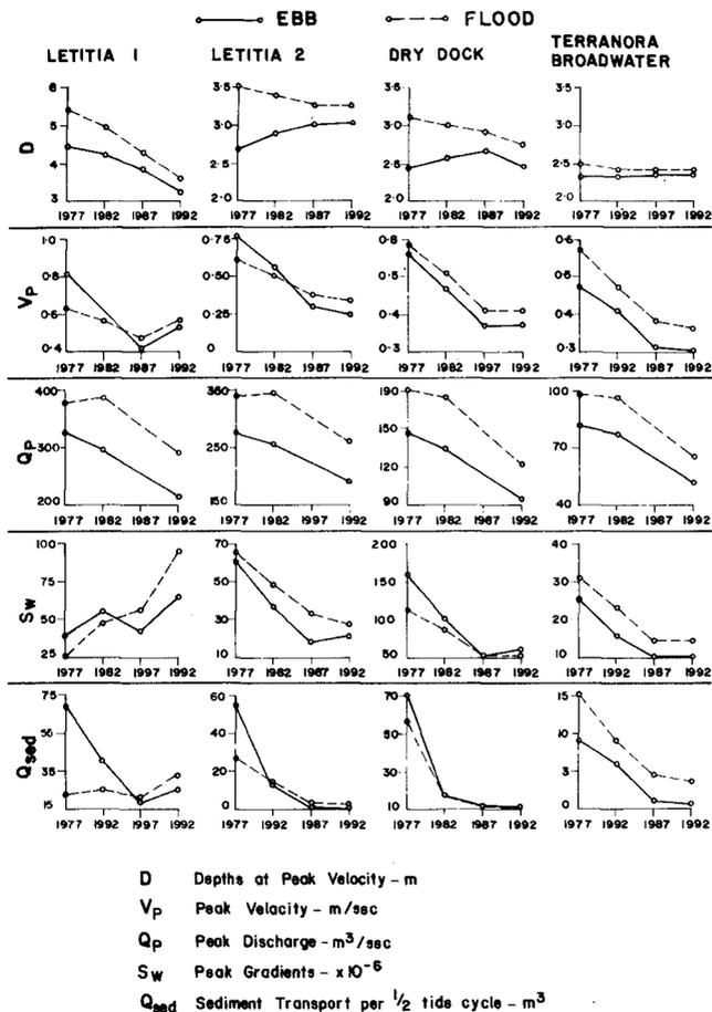
Figure 16 Variation of Hydraulic Parameters Due to Shoaling
