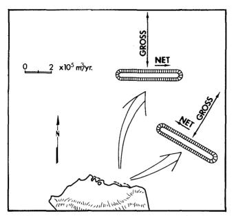
Figure 5. Sediment transport rates on hypothetical deep-water artificial islands.
