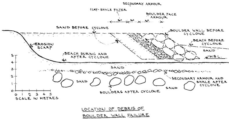
FIGURE 4. Location of Debris of Boulder Wall Failure.
