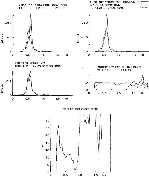
FIG.4 SEPARATION OF INCIDENT AND REFLECTED SPECTRA
