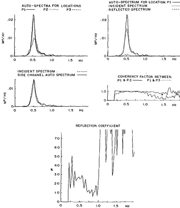
FIG. 3 SEPARATION OF INCIDENT AND REFLECTED SPECTRA
