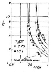
Fig. 7 Comparison of wave celerity with theoretical curves
