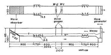
Fig. 4 New wave flume used
