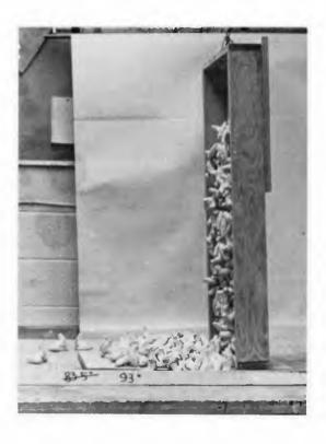
Figure 1 - Totally Stable up to 91° 80% of Dolos Units Stable at 93°
