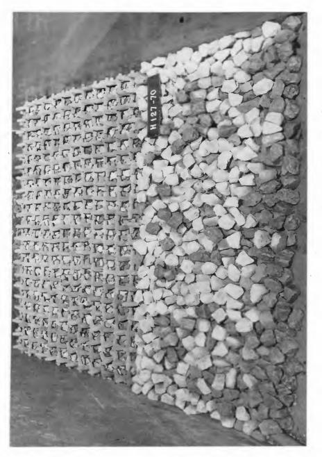
Photograph 4. Pattern 2 with one layer of armor units in place
