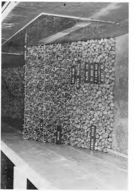
Photograph 3. Pattern 1 after attack of 2.65-sec, 18.5-cm waves
