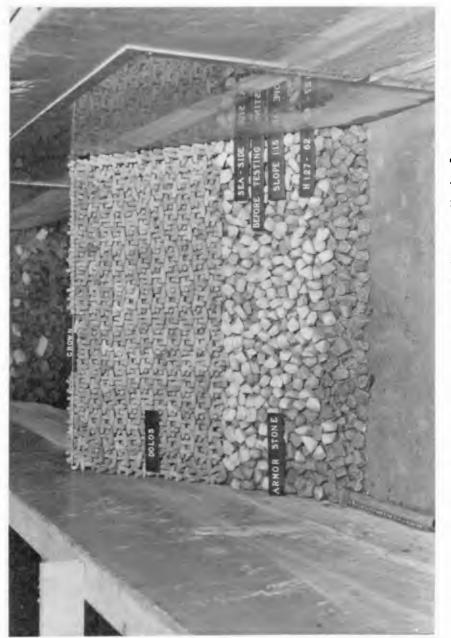
Photograph 8. Pattern 3 with two layers of armor units in place
