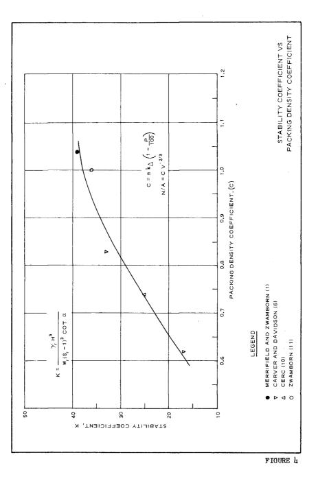
References (1) and (11) are based on 2 percent damage by number of displaced units. These data do not necessarily recommend an optimum number of dolosse to use per given area because the safety and economics of each prototype project should be considered on its own merits. They do show, however, that the number of dolosse used per given area is critical to the selection of the stability coefficient and should be considered accordingly.
