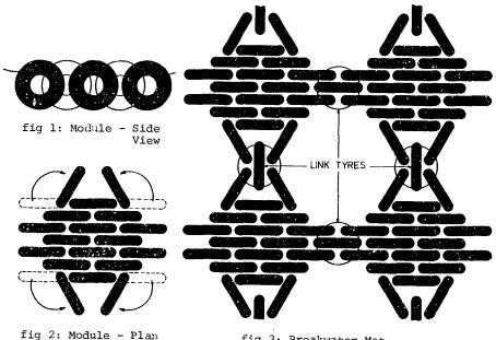
fig 3: Breakwater Mat
