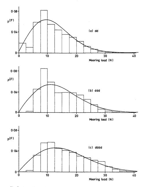
fig 7: Comparison of Mooring Load Histogram with Rayleigh Distribution
