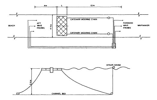
fig 4: Experimental Arrangement
