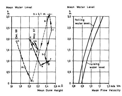
Fig. 8 Mean Dune Height, Flow Velocity and Water Levels in the Rio Paraná (STÜCKRATH, 1969)
