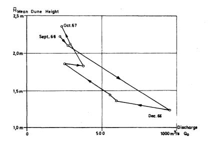
Fig. 3 Mean Dune-Height Discharge Curve for River Weser
