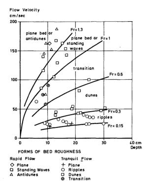
Fig. 6 Flow Velocity, Water Depth and Bed Form (SIMONS and RICHARDSON, 1960)
