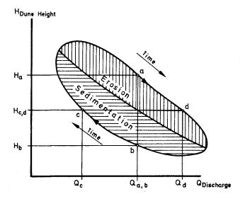
Fig. 4 Schematic Dune-Height Discharge Curve for River Weser
