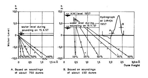
Fig. 7 Dune Heights on the Niger at Low Water and at High Water (NEDECO, 1959)
