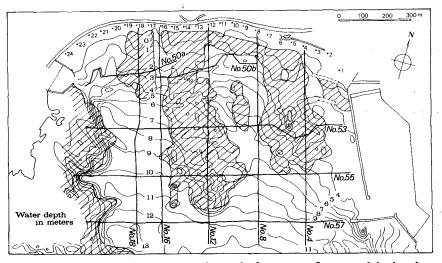
Figure 3 Submarine topography and the area of exposed bedrock (hatched area).
