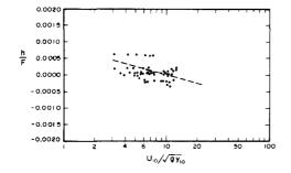
Figure 16. Surface set-up as a function of Froude number
