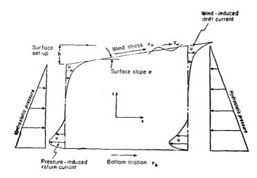
Figure 1. Free-body forces diagram
