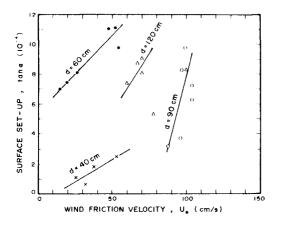
Figure 15. Relation between surface set-up and wind friction velocity at fetch 22<sup>m</sup>
