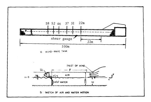
Figure 2. Sketch of wind-wave tank and air-water motions
