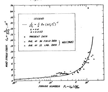
Figure 4. Froude number scaling of wind stress coefficients
