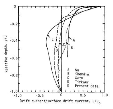
Figure 11. Comparsion of drift current profiles
