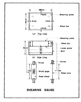
Figure 3. Shear gauge
