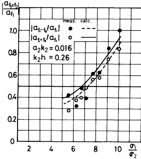
Figure 5. Comparison of calculated amplitudes of waves produced by second order interaction and experimental results (1)
