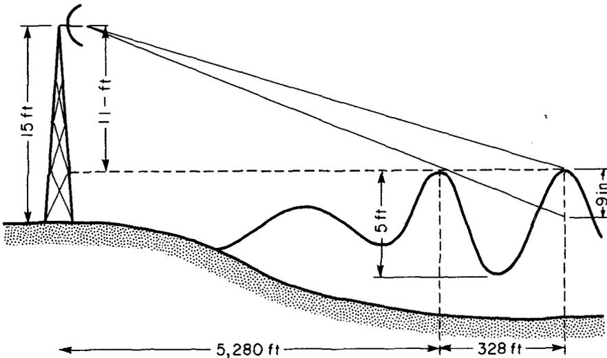
Figure 5. Illustration of the shadowing of a portion of one wave, by a wave nearer to the radar.
