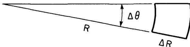
Figure 6. Resolution cell for the radar image.  $R$  is the range,  $\Delta R$  resolution along the radar beam.  $\Delta R = c\Delta T/2$ , where  $c$  is the speed of light and  $\Delta t$  is the duration of a radar pulse.  $\Delta\theta$  is the azimuthal resolution.
