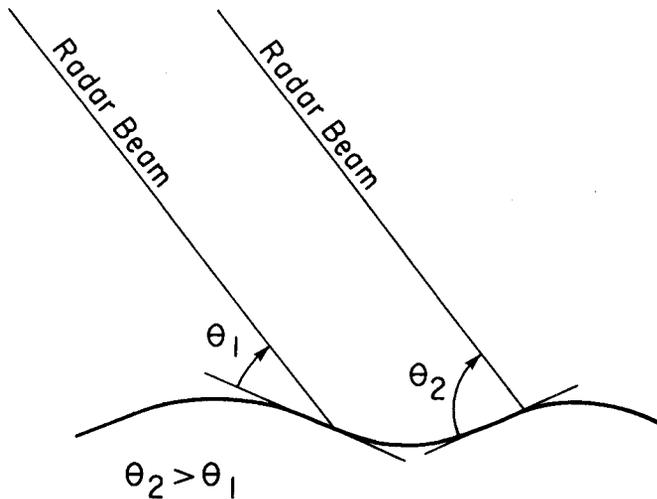
Figure 4. Modulation of the incident angle of the radar beam by the long waves.
