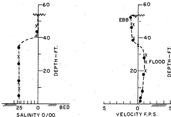
Fig. 3. Comparison of Model (x) and Prototype (o) 2.2 Hours after Low Tide
