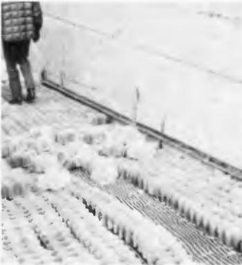
Figure 4. Gobi blocks in the large wave tank at CERC
