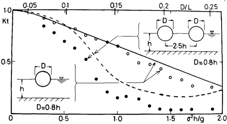
Fig.3-3 Transmission Coefficient of Single and Double Cylinders
