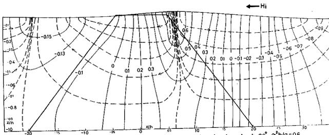
d Distribution of Velocity Potentials for Type A Breakwater at  $\alpha t = 90^\circ$ ,  $\alpha^2 h/g = 0.6$
