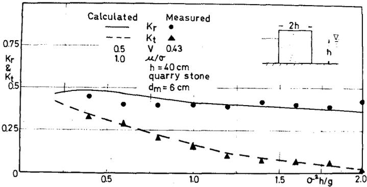
Fig. 5-6  $K_r$  and  $K_t$  for Vertical-Face Breakwater
