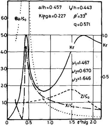
Fig. 4-3 Amplitude of motions and Reflection coefficient
