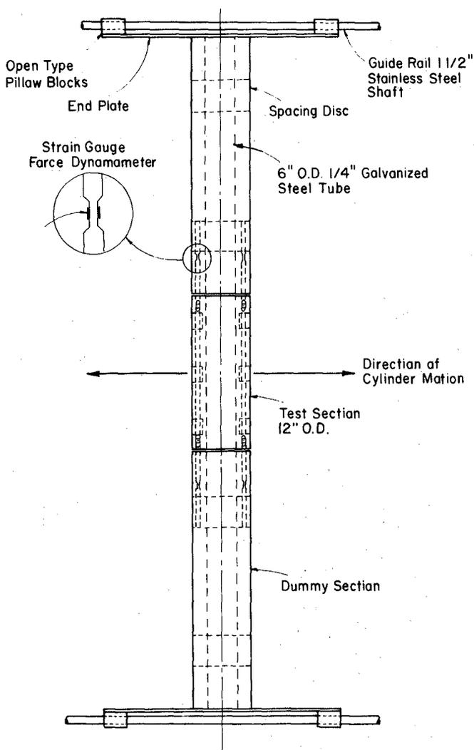
FIG. 2 Test cylinder for Forced Cylinder Oscillation Tests.
