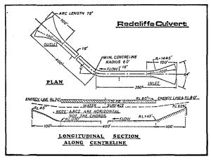
FIG.2. DETAILS OF REDCLIFFE CULVERT
