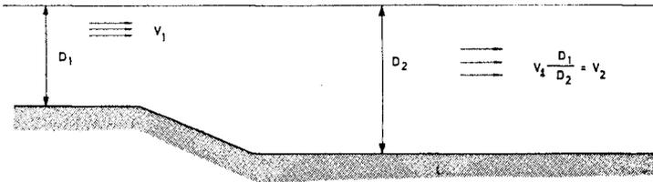
The undredged depth is called  $D_1$ , and the corresponding current velocity  $V_1$ . The depth in the channel is called  $D_2$  and the corresponding current velocity  $V_2$ .
