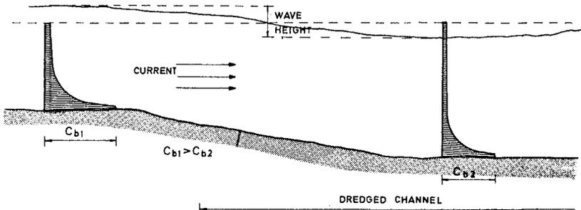
As the flow passes the side of the channel, its velocity changes and therefore the total sediment load, carried as bed load and suspended load, changes accordingly.
