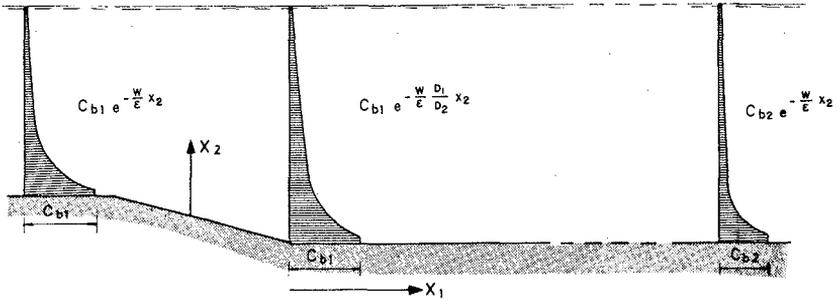
At the toe of the side slope of the channel the approximation is made that the bottom concentration is unchanged, but the concentration profile is stretched with the same ratio as the depth is changed, i.e.  $\frac{D_1}{D_2}$ . Therefore the concentration is given by
