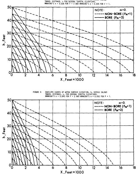
ENVELOPE CURVES OF WATER SUBFACE ELEVATION, h, VERSUS INLAND TRAVEL DISTANCE, x FOR SEVERAL COASTAL ELEVATIONS. MANNING'S n = 0.035 FOR F = 2 ANO MANNING'S n = 0.025 FOR F = 1. FIGURE 3
