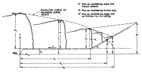
FIGURE 1 SCHEMATIC DIAGRAM OF BORE ADVANCEMENT AND DEFINITION OF SYMBOLS
