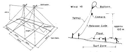
Fig. 1 Schematic diagram of SIHELS. Fig. 2 Schematic diagram of BACS. (Horikawa and Sasaki, 1972)
