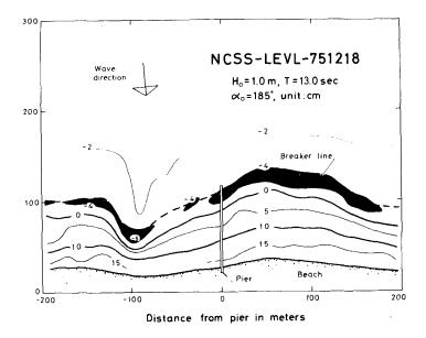
Fig. 12 Simulated mean water surface elevation.
