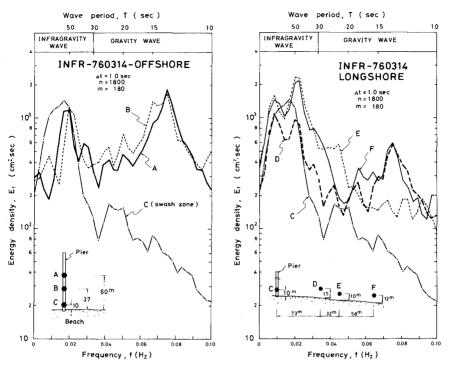
Fig. 17 On-offshore infragravity Fig. 18 wave spectrum (March, 1976).
