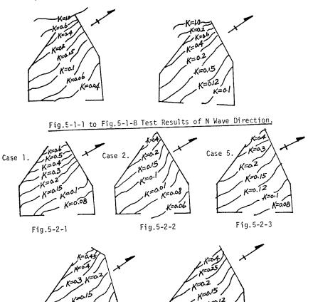
Fig.5-2-1 to Fig.5-2 -5 Calculated Diffraction Diagram.
