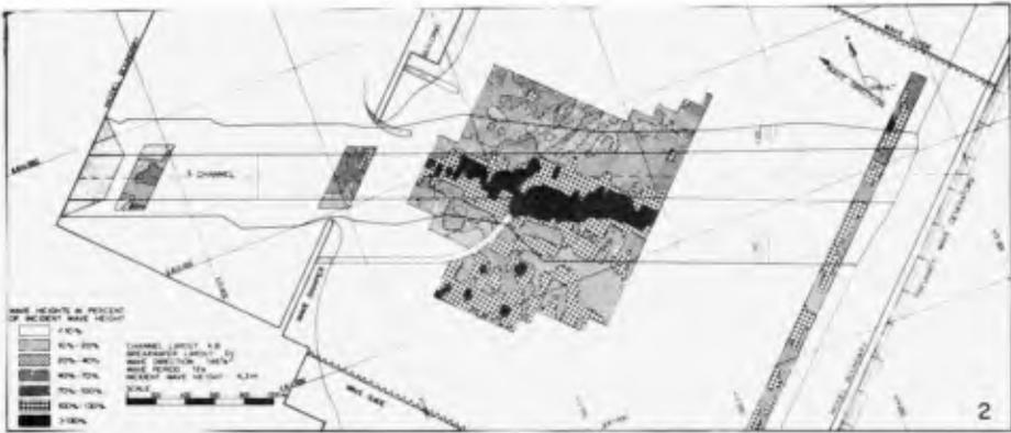
Fig. 10. Wave penetration diagram, 1:60 slope,  $146\frac{0}{4}$ , 12 s waves.
