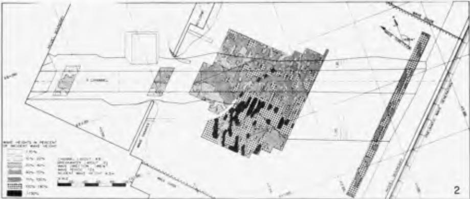
Fig. 11. Wave penetration diagram, 1:100 slope,  $146\frac{0}{4}$ , 12 s waves
