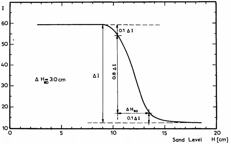
Fig.5. Resolution for water-sand contact.
