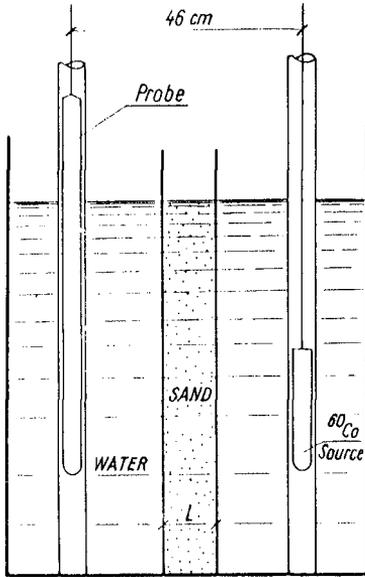
Fig.3. Tank for probe calibration.
