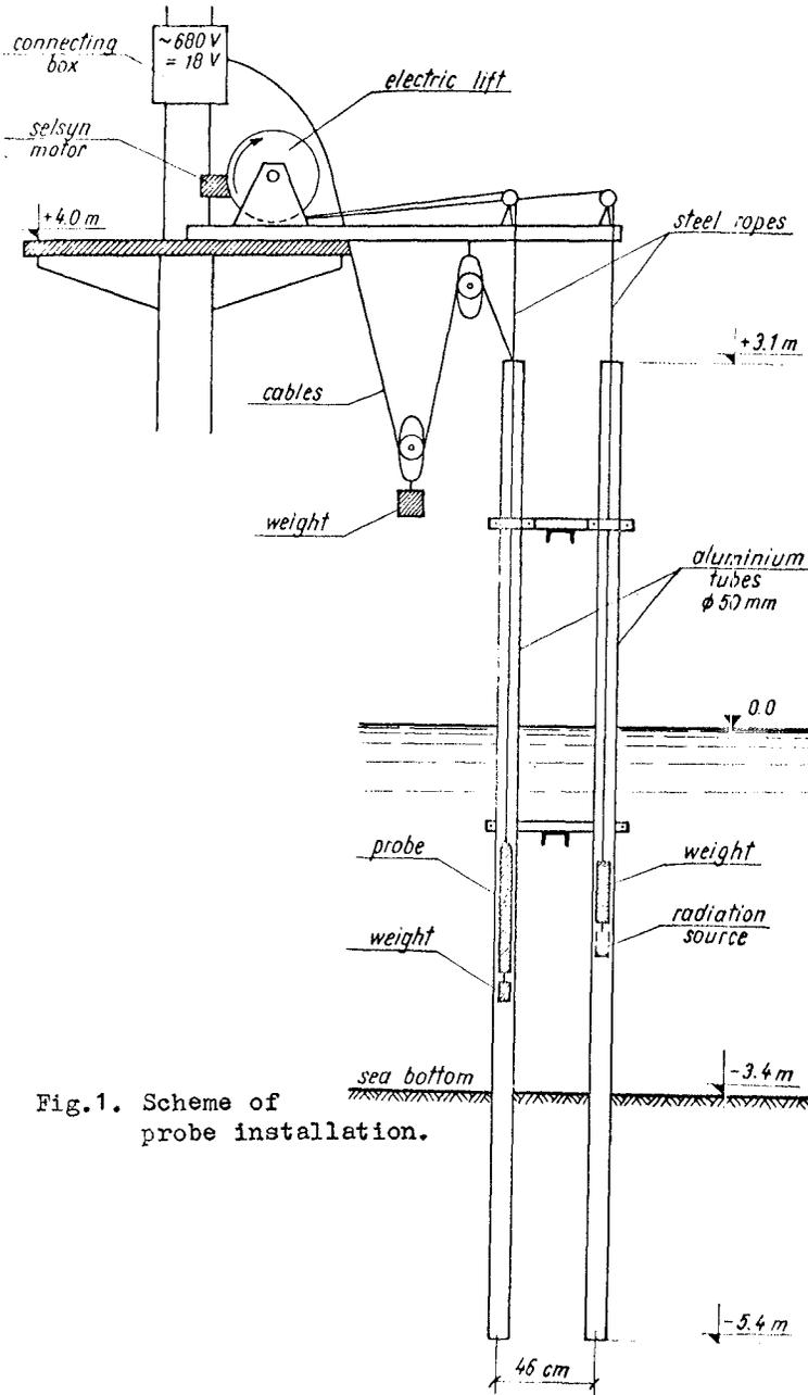
Fig.1. Scheme of probe installation.
