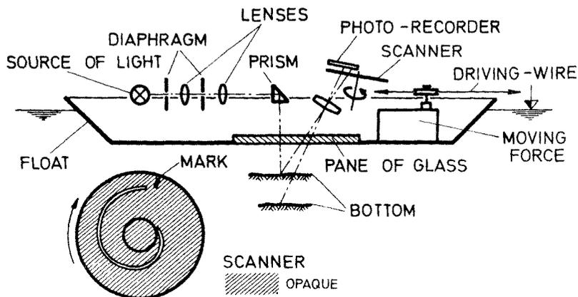
Fig. 8 Optic-electrical recording instrument for morphological sounding
