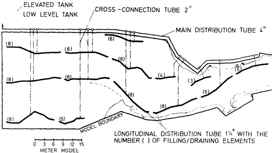
Fig. 7 Distribution system for irrigation and draining
