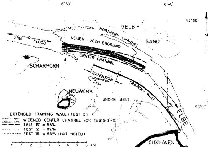
Fig. 16 Changed positions of the "Center Channel"
