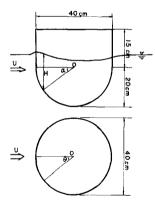
Fig. 6. Circular Cylindrical Type Buoy Fig. 7. Pressure Distribution on with Hemispherical Bottom
