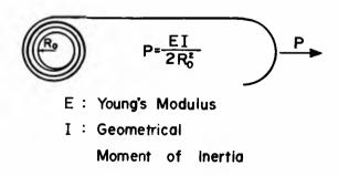
Fig. 9. Special Coil Spring with Constant Reaction
