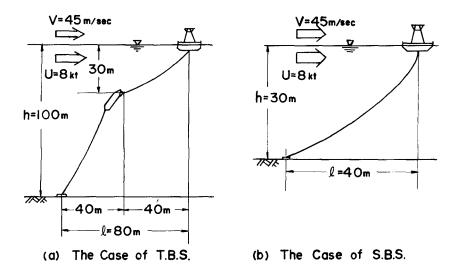
Fig. 3. Fundamental Plans of Mooring System
