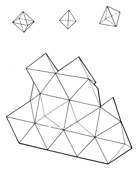
Figure 5. Regular polyhedra will pack to fill space in a complimentary manner. When space is filled in this manner, such as in the formation of a groin, the efficiently spaced ligaments (formed by the equilateral triangles that are the original boundaries of the shapes) have excellent resistance to internal shear.
