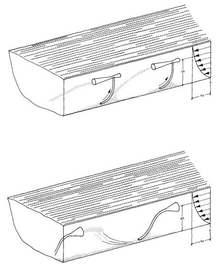
Figure 4. Cascade methods of enhancing sediment transportation need study to capitalize on difference in velocity potential in a fluvial system or in a harbor entrance. Tethered, buoyant units could capture the maximum velocity compatible with maximum ship depth and assist in channel maintenance without placing claims upon the earth's energy budget.
