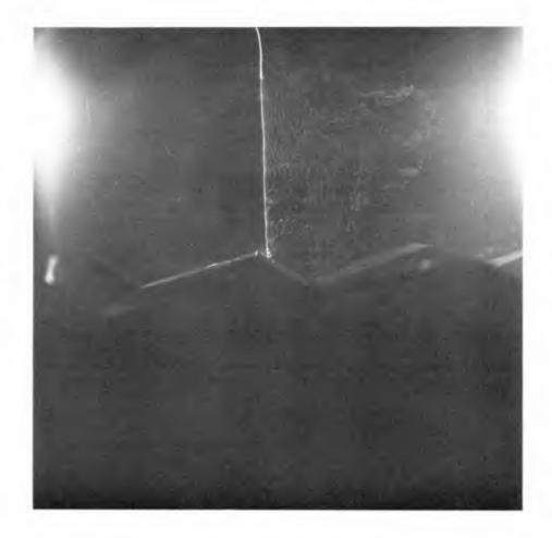
Figure 5. Large vortex formed over steep side of asymmetrical roughness element. Wave form travels from left to right.
