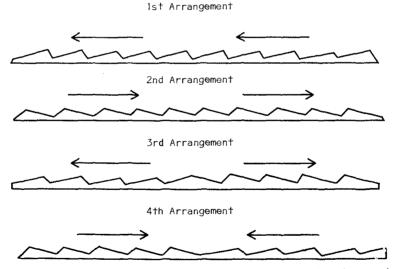
Figure 4. Laboratory demonstration of the capability of phase dependent roughness elements to control the direction of sediment transport. In each case the wave traveled from left to right.
