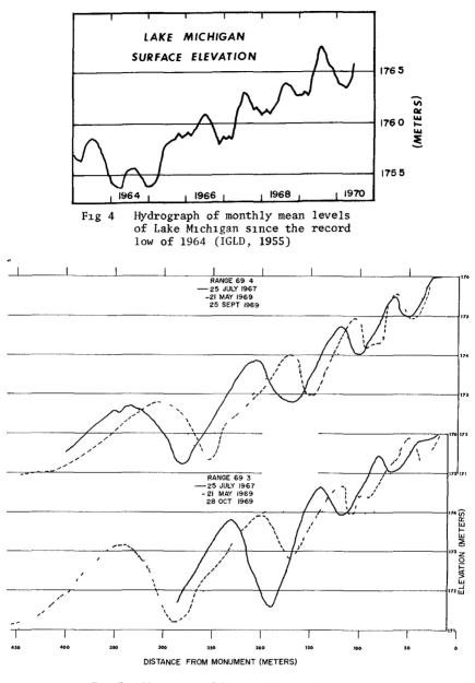
Fig 5 Movement of bars and troughs
