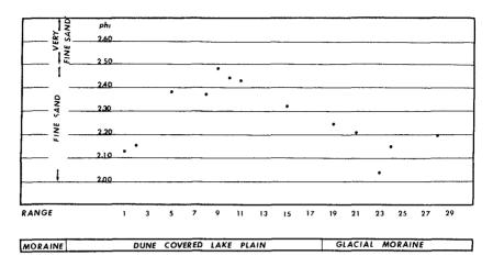
Fig 8 Longshore variation in mean diameter of mobile sediment
