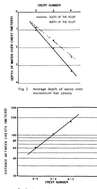
Fig 3 Average distance between bar crests based on measurements at 29 sites over approximately 45 km
