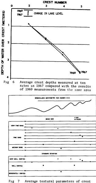
Fig 7 Average textural parameters of crest and trough samples from ranges 9-13 Trough samples are coarser and more poorly sorted than samples from adjacent troughs These observations are in accord with the principal theories on bar genesis, in as much as the various theories all envision some winnowing action at trough sites with concomitant deposition on a bar site located immediately lakeward
