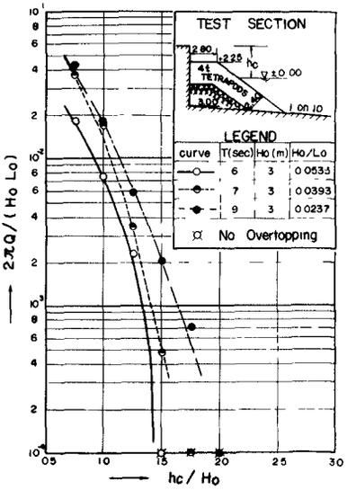
Fig. 3-a,  $h/H_o = 1$  Relation between  $2\pi Q/(H_o L_o)$  and  $hc/H_o$  with a parameter of  $H_o/L_o$
