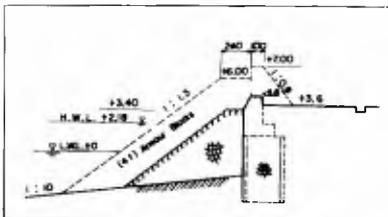
Fig. 15 Cross section of seawall at Beppu Coast. Dotted line is the section of plan to prevent the wave overtopping after the damage at Typhoon No.9.
