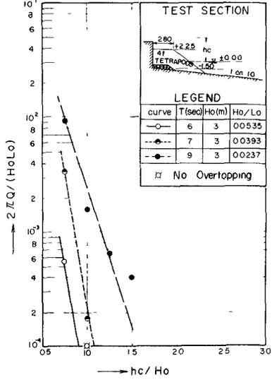
Fig. 2-a,  $h/H_o = 0.5$  Relation between  $2\pi Q/(H_o L_o)$  and  $hc/H_o$  with a parameter of  $H_o/L_o$
