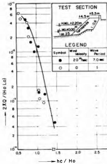
Fig. 14 Experimental results of wave overtopping at Oita Coast.
