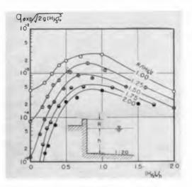
Fig. 12 Expected overtopping discharge on vertical wall
