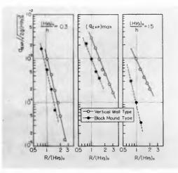
Fig. 14 Sea wall height for a given discharge of irregular wave overtopping
