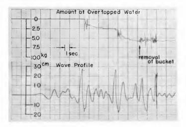
Fig. 4 Sample record of wave overtopping and wave profile
