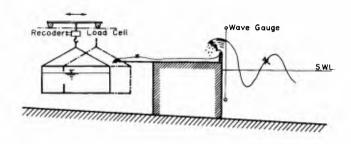
Fig. 3 Experimental set-up for the measurement of wave overtopping
