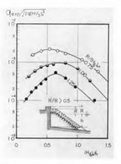
Fig. 13 Expected overtopping discharge on sea walls covered with concrete blocks.
