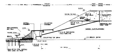
FIG 1 SECTION THROUGH THE CLIFF SHOWING THE DRAINAGE SYSTEM
