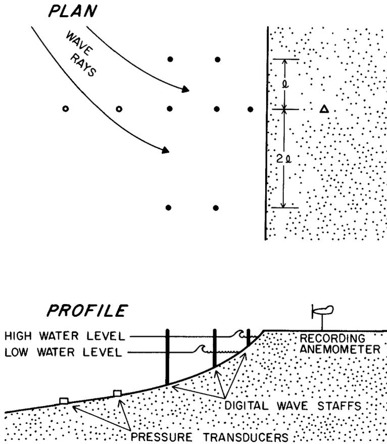
Figure 1. Schematic diagram of sensor array used for measuring direction and flux of wave energy (after Koontz and Inman, 1967, Fig. 16) Cross-spectral analysis shown in Figure 2 is from a longshore pair of such an array.
