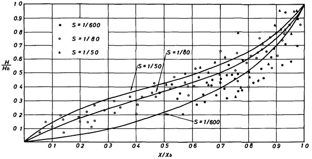
Fig. 7. Wave height after breaking.
