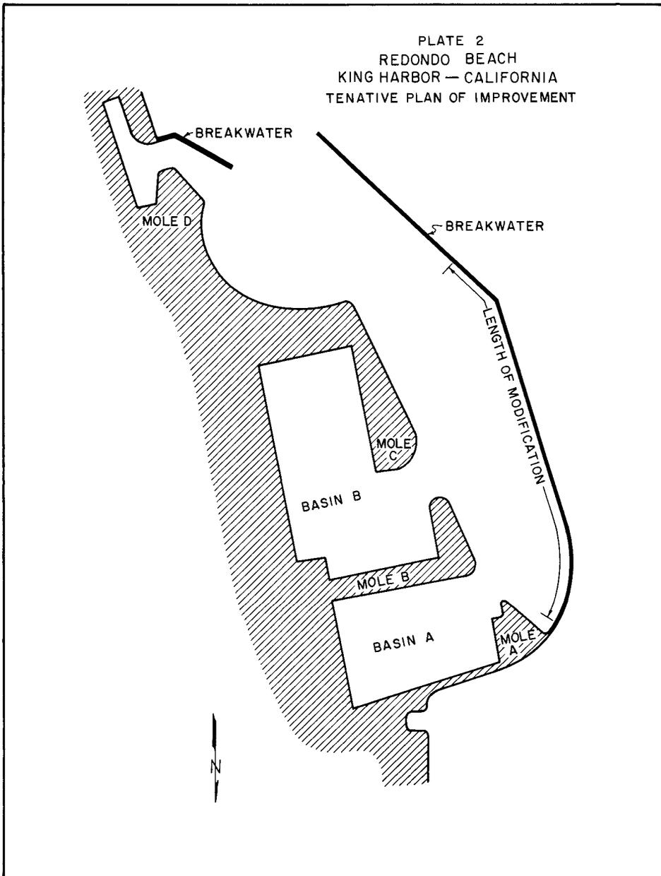
knowledge of the actual characteristics of the waves impinging on the harbor, the degree of energy transferred through the voids, and the degree of wave reformation resulting from overtopping were not fully considered. Design of a modification included hydraulic model study, which was accomplished during the fall of 1963.
