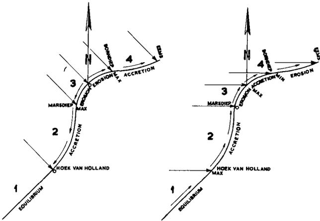
Fig. 3. Effect of waves on the Dutch coast-line.
