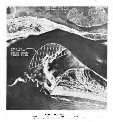
AERIAL PHOTOGRAPH, FIRE ISLAND INLET, N.Y. TAKEN 12 SEPTEMBER 1955 AT TIME OF LOW WATER Fig. 9. Phase 1 of "Alternative Short Range" plan.
