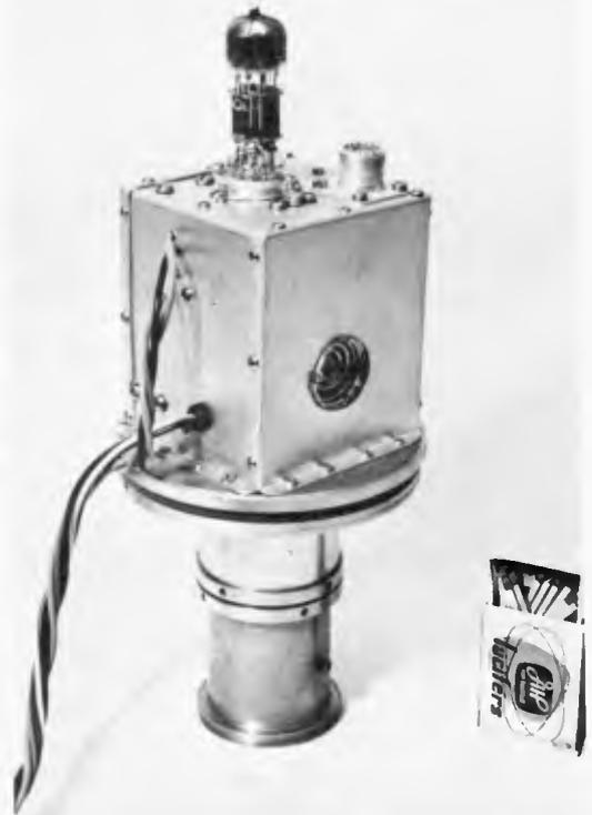
Fig. 4. Construction of the accelerometer. Fig. 5. Transmitter on top of accelerometer.
