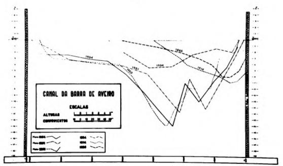
Fig. 29. Evolution of the inlet's channel crosssections due to the works (range No. 11).
