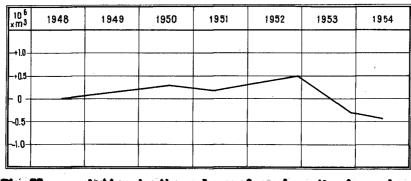
Fig 32 variation in the volume of sand on the inner bar from 1948 to 1954.
