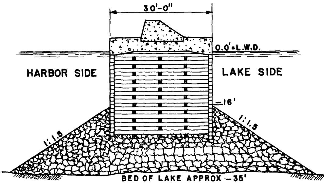
Fig. 3. Cross-section of Gary breakwater
