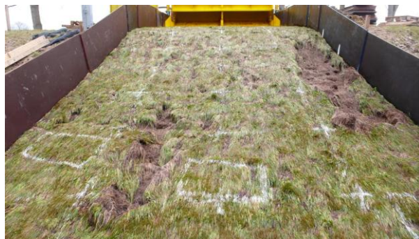
Figure 24. Damage section V3 after test session 30 l/s per m
