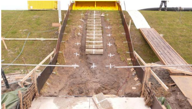
Figure 16. End result test section A3 after 2 hours 75 l/s per m
