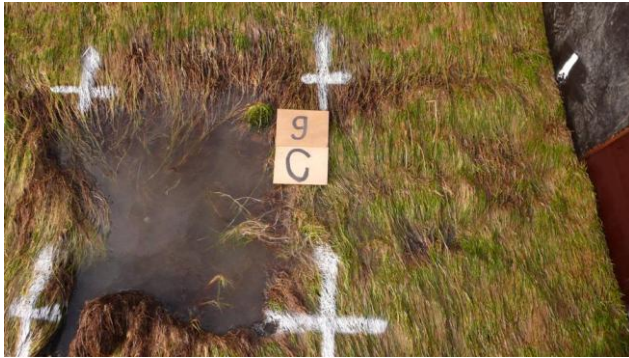
Figure 9. Initial damage at toe of section 1 ( 0.75 \text{ m}^2 ; depth 0.1 \text{ m} )
