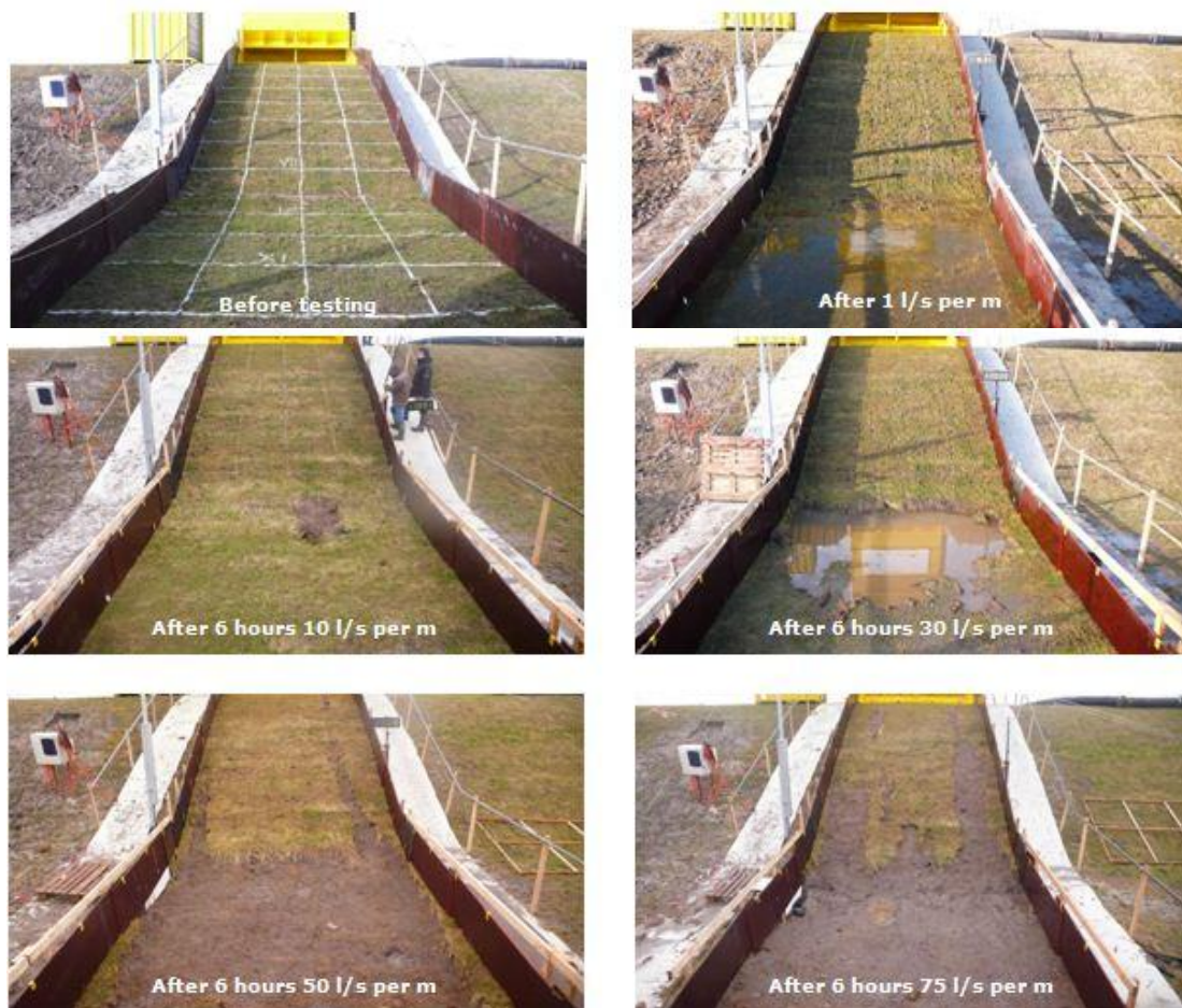
Figure 10. Development of damages in test section 1
