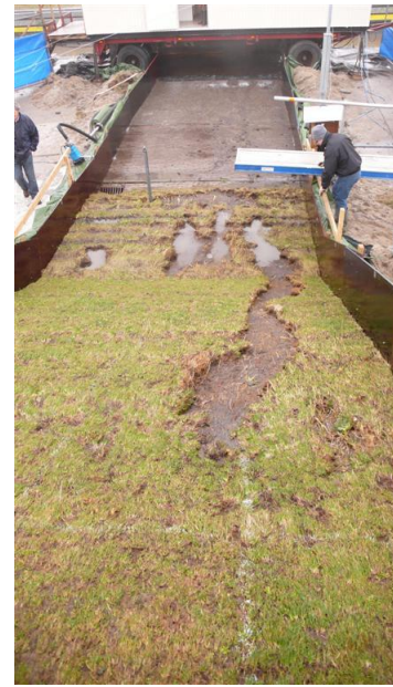
Figure 11. Damage section A2 after 6 hours 10 l/s per m
