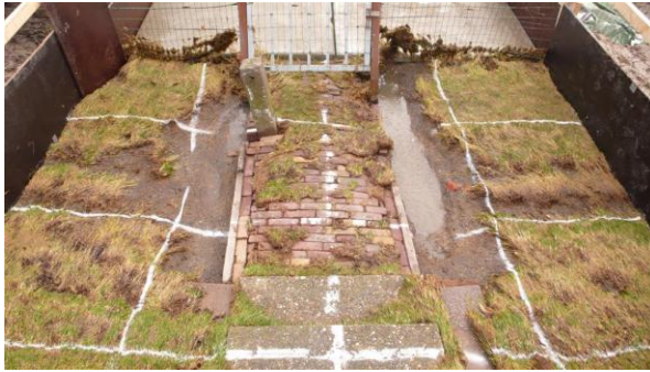
Figure 14. Result after 6 hours of 10 l/s per m.
