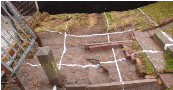
Figure 15. Result after 4 hours of 30 l/s per m.
