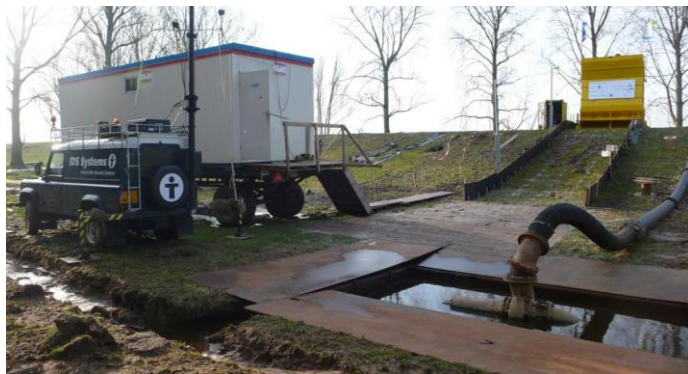
Figure 5. Set up of overtopping tests at the Vecht dike
