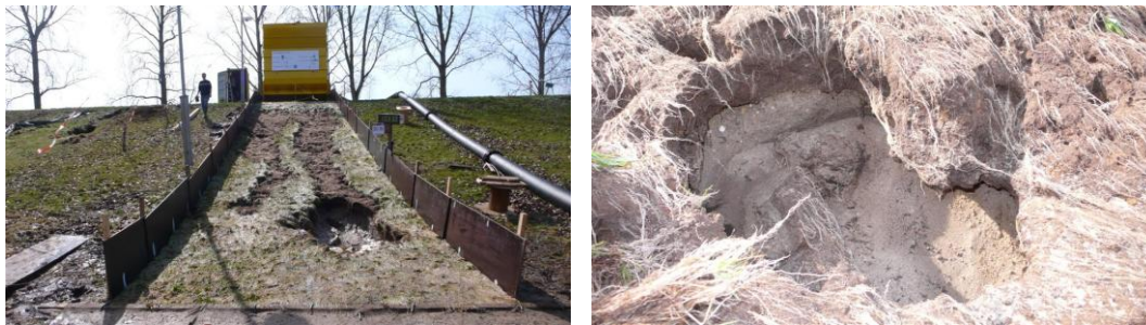
Figure 26. End result section V4 after 1 hour 30 l/s per m
