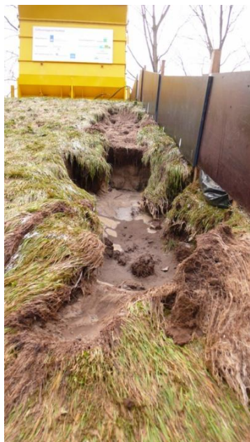
Figure 25. End result section V3 after test session 50 l/s per m
