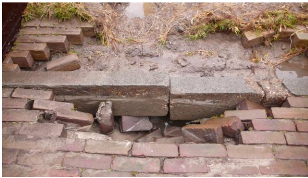
Figure 12. After 4 hours 30 l/s per some bricks of the parking lot were removed
