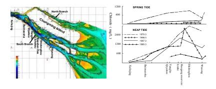
Figure 2. Distribution of Chloride Along the Route
