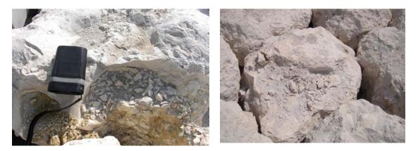
Figure 2. Examples of rocks showing surface crumbling after approximately three years in service.
