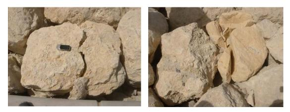
Figure 3. Examples of rocks which have been broken during placement.
