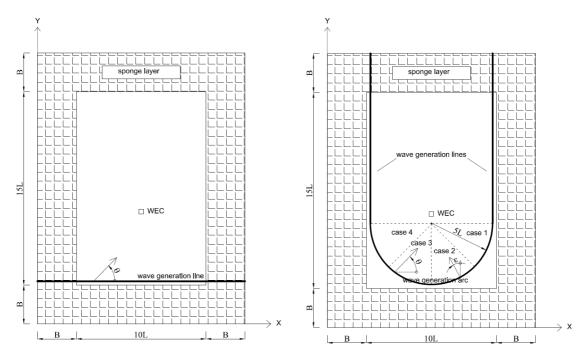
Figure 1. Definition sketch of wave basin in plan view for generation of long-crested waves.
