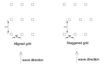
Figure 5. Aligned and staggered grid lay-out.
