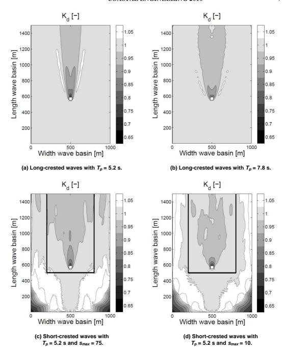
Figure 4. Calculated disturbance coefficient  $K_d$  in a wave basin with a single WEC (capture ratio = 45 %) for irregular long-crested waves (head-on) with respectively  $T_p = 5.2$  s (a),  $T_p = 7.8$  s (b) and for irregular short-crested waves (head-on - useful domain indicated with black lines) with  $T_p = 5.2$  s and respectively  $s_{max} = 75$  (c),  $s_{max} = 10$  (d).
