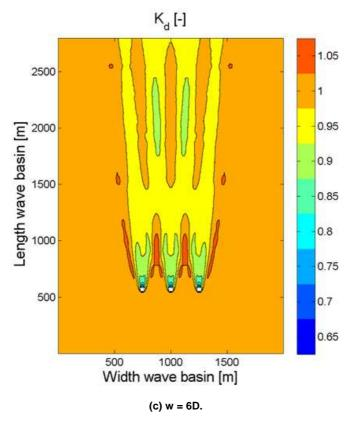
Figure 7. Calculated disturbance coefficient  $K_d$  in a wave basin with 3 hypothetical WECs with an in-between distance of respectively (a) 2D, (b) 4D, (c) 6D with D = 36 m for irregular long-crested waves (head-on) with  $T_p$ = 5.2 s.
