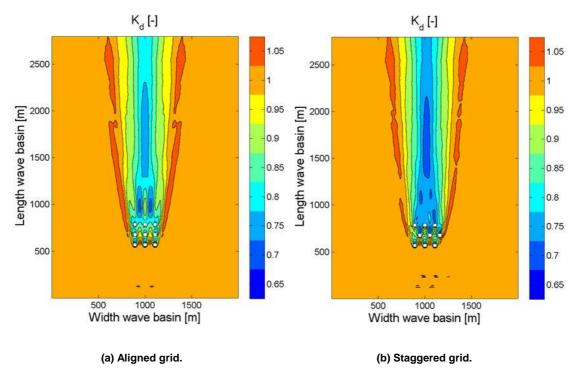
Figure 8. Calculated disturbance coefficient  $K_d$  in a wave basin with 9 hypothetical WECs with an inbetween distance of 2D with D = 36 m for irregular long-crested waves (head-on) with  $T_p$  = 5.2 s.
