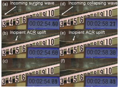
Figure 7. ACR structural response under wave loadings for configuration A3F9. A surging wave approaches from the left (panel (a)), impacts the structure, inducing ACR motion (panel (b)), and runs up the ACR with continued mat displacement (panel (c)). Similarly, a collapsing wave approaches from the left (panel (d)), impacts the structure, inducing ACR motion (panel (e)), and runs up the ACR with continued mat displacement (panel f).
