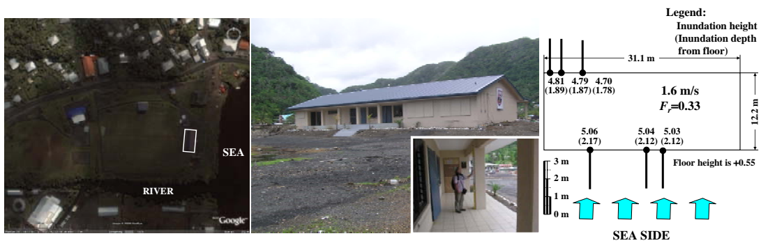
Figure 7. Tsunami-trace heights and their distributions around buildings in Tutuila Is., American Samoa in the 2009 Samoa Earthquake tsunami.
