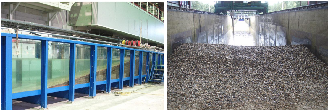
Figure 2. Small-scale (left) and large-scale (right) wave flume tests.
